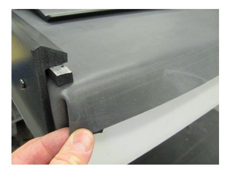
...butt the two edges together with overlapping tapes and attach.
