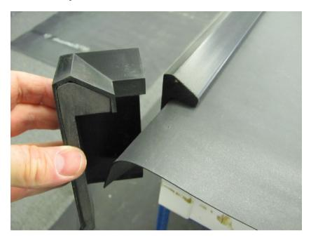
When joining two lengths of Permaroof Plus kerb edge trim, use a joint clip. Have at least 5mm between both trims and the joint clip to allow for expansion.
