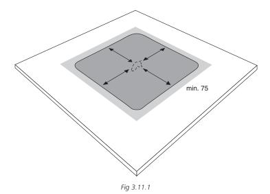
Cuts and punctures in the EPDM membrane should be repaired with cured membrane. Round all edges of the cut so that it cannot propagate underneath the target piece. If this has been done properly, the target EPDM repair piece can be applied using QuickSeam Tape and QuickPrime Plus. A valid alternative is to fully adhere a piece of QuickSeam SA Flashing using QuickPrime Plus.
