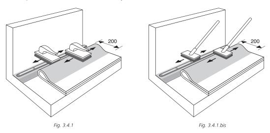
Remove the release paper from the Q.S.R.P.F. Strip and roll the field membrane toward the change of angle, keeping a rounded leading edge to avoid wrinkles. Hold both hands on top of the coated membrane when rolling it in, to avoid bridging in the change of angle.
