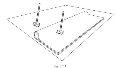
The EPDM-sheets are to be fully adhered with Bonding Adhesive. Stir the Bonding Adhesive before and during application to achieve a uniform mix with no sediment at the bottom. Properly mixed adhesive is critical for desired performance and uniformity of the bond.
