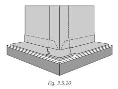
Repeat this procedure, starting from the other side to provide an overlap of at least 75 mm at the corner. Apply QuickPrime Plus on the area to be overlapped, complete the corner detail and seal all exposed cut edges of the QuickSeam FormFlash with Lap Sealant.
