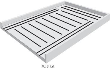
A continuous row of QuickSeam R.M.A. strips shall be installed along the inside edge of the perimeter sheets, to separate the perimeter zones from the central zone of the roof.
