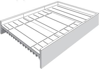
Prior to installing the batten strips over the sheets, make sure that the EPDM panels lay smoothly without any wrinkles and remove excess dirt and moisture from the membrane. Use a chalkline to mark the correct position of the batten strips as per layout and make sure the strips are positioned in straight lines.
