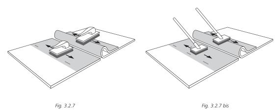
Apply the QuickPrime Plus using long back and forth scrubbing strokes, parallel to the seam along the length of the splicing area, until the surface becomes dark grey in colour with no streaking or puddling. Scrub both surfaces at the same time to allow the same flash off time, start on the folded overlap. Make sure to overlap the guide marks on the bottom sheet and go beyond the edge of the top sheet.
