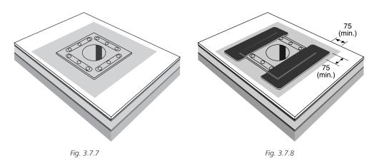
Roll the QuickSeam FormFlash/SA Flashing cover pieces with a 50 mm silicone rubber roller and seal all exposed cut edges.
