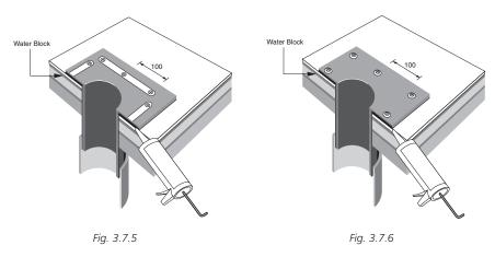
Apply QuickPrime Plus to the designated area. The flange is flashed-in with QuickSeam FormFlash strips or a piece of QuickSeam SA Flashing extending 75 mm onto the field membrane and 75 mm past the fasteners in all directions.
