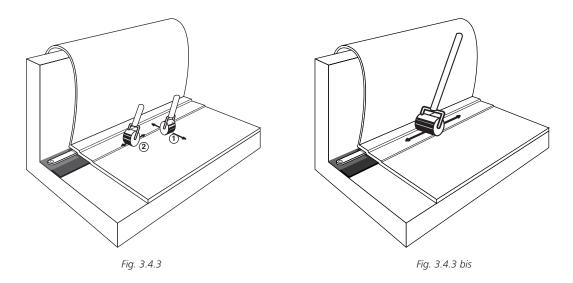
Apply Bonding Adhesive simultaneously to both wall and backside of the field membrane to allow for equal drying times. Apply the adhesive first to the wall to avoid spilling adhesive over a surface that has already been covered.
