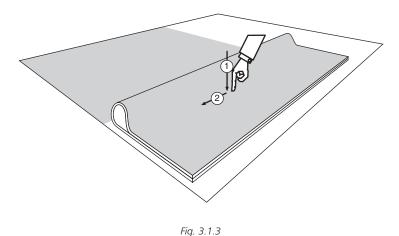
Push forward on the adhesive at an angle to ensure that it is dry throughout its thickness. If either motion exposes wet or stringy adhesive when the finger is lifted then it is not ready for mating.
