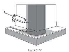
The one-piece outside corner detail cannot be executed in regular FormFlash using Splice Adhesive. An outside corner detail in regular FormFlash always requires the use of 2 pieces (see hereafter).
