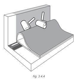
Allow the adhesive to dry. Once the adhesive has flashed off, roll the flashing up the vertical surface. Keeping a rounded leading edge will result in a wrinkle free application. When the flashing is installed by two people, the operation should be started in the centre, working out towards both ends. Roll the flashing evenly into the adhesive. Work slowly up the wall, mating the flashing to the substrate by hand. Compress the bond with a stiff brush.
