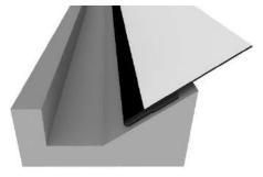
Install RubberGutter EPDM SA without any tension and avoid entrapment of air.
