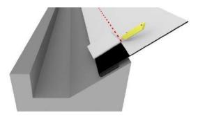
Fold the membrane back in position, remove the second part of the release liner and adhere the membrane till the angle change.
