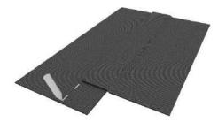
• Fold back the top membrane and mark the bottom sheet every +/- 10 cm at 10 mm from the marked edge (at the side of the overlap).
