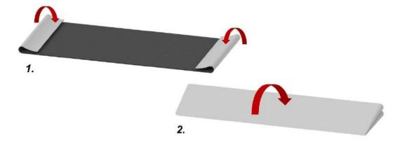
Once the membrane is in position, flap back the edge from the inner or outer side of the gutter and cut the plastic release liner approx. 50 mm from the edge without damaging the membrane.
