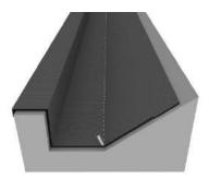
• Flap back the membrane to the other side with ply at first angle-change. Cut the release liner also here without damaging the membrane.
