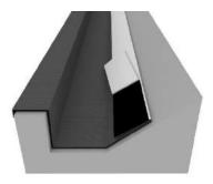
Remove the release liner and stick the membrane to the substrate.
