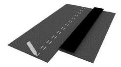
• Clean the seaming area with a damp rag and apply a continuous line of EasySealant over the marks (10 mm from the seam edge) at a speed of +/- 6 sec/10 cm (min. 6 mm bead width) while the membrane is still damp (not wet).
