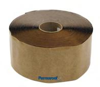
Cured EPDM flashing tape. Cannot be used as a detailing tape.
