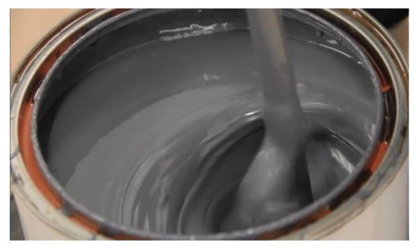
Add the accelerator and mix again with a low-speed mixer for a couple of minutes until completely blended.
