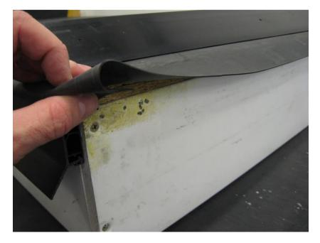
...offer the trim into place and fix securely. There are pre-drilled 7mm slots every 300mm down the length of the trim for easy fitting.
