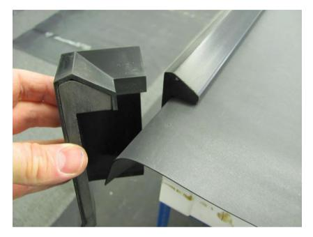
When joining two lengths of Permaroof Plus kerb edge trim, use a joint clip. Have at least 5mm between both trims and the joint clip to allow for expansion.
