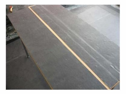
**Step 6:** Flap the leading edge back, and check the distance to the brown paper edge of the tape. This should be around 18mm. Trim the top leading edge if necessary.
