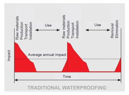
Due to their larger mass and shorter life span, **bitumen membranes have a more significant environmental impact (GWP)** during production, transportation and installation.
