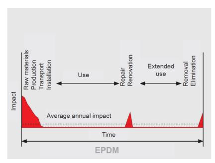
EPDM membranes have a longer life span and as they are easy to repair, meaning that complete renovation of the roof which is usually high in  $CO_2$  emissions can be delayed.
