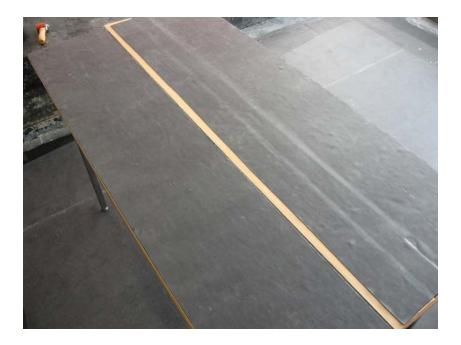
Lift up the leading edge, and starting from one end of the tape, peel the backing paper towards you, and let the primed leading edge fall onto the tape, flattening down with your hand whilst peeling.
